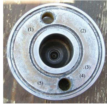
Fig. 6. The hardness measurement points
